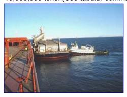
Vessels are loaded by means of two purpose-built barges which are operated by Foss Maritime of Seattle, each barge being capable of carrying a quantity of 5,443 metric tons and typically making two round trips per day, so that, under normal conditions, the average rate of loading is in the region of 20,000 tons per day.
