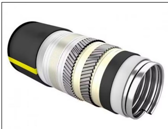
Figure 6: Hybrid Flexible Riser cross section. Courtesy of 2Hoffshore
